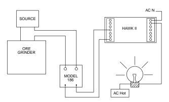
Time delay should be set at 1, which will allow the load to exceed 25 amps for one second before activating the relay.
