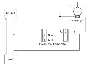
Time delay should be set at 2, allowing the current to rise above the alarm set point for two seconds before the relay is energized.
