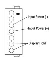
**Supply Power:** Connect the appropriate power to the **supply power** terminals.
