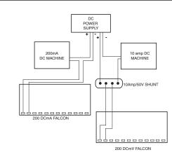
The shunt is installed in series between the source and the load, and the meter is connected to the shunt in parallel. The two lead wires included with the shunt are connected to terminals #1 and #2, located on the rear of the Falcon. Be sure to place a jumper across R114 when using a 10 amp/50mV shunt.
