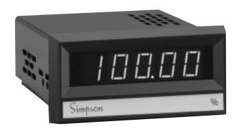
Simpson's 2842 Series meters take in a 4-20mA signal and display 0-100.00%. Model 2842 requires a 117VAC input at 50-400Hz. The large 4-1/2-digit display is easily read from a distance of about 25 feet. Panel adapters are available for 1/8 DIN panel cutouts. In addition, a large "U" shaped mounting bracket is available for applications where the panel strength is unknown or weak.
