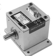
To aid in troubleshooting, LEDs are located directly on the body to instantly verify correct output operation. Quadrature output is standard and can be externally scaled to provide any engineering unit (RPM, angular position, feet/min., etc.). Gold-plated connectors ensure maximum signal transfer. Very low power consumption; typical current draw, 35mA @ 15DCV.
