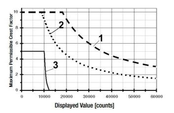
Additional error caused by signal's crest factor: 1 < CF < 3: 1% R + 30D 3 < CF < 10: 3% R
