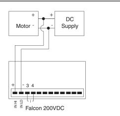
dard feature on the Falcon. By shorting connections #3 and #4, the operator can hold the display to take a reading, and then remove the short to reactivate the indication mode. A switch can be used to short the connections. The meter is shipped ready to install, keeping down-time to a minimum.
