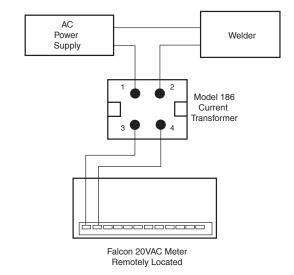
The current transformer is installed in series between the power supply and the welding process. The Falcon AC volt meter is connected to the transformer.
