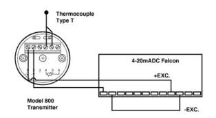
located to the right of the display, until the meter indicates 100.0 (degrees). Carefully put the bezel back on the meter. Remove the signal input. The Falcon has an optional 12 or 24VDC excitation output to power the transmitter, eliminating the need to mount an external DC power source for the transmitter.
